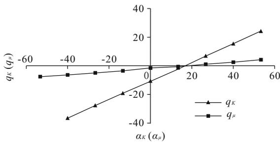
**Figure 5.** The curves of change rates of estimated groundwater withdrawal ( $q$ ) with the rates of hydraulic conductivity  $\alpha_K$  and specific yield  $\alpha_\mu$ .
