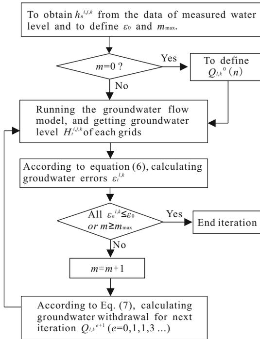
**Figure 1. Flow chart of groundwater withdrawal inversion analysis.**
