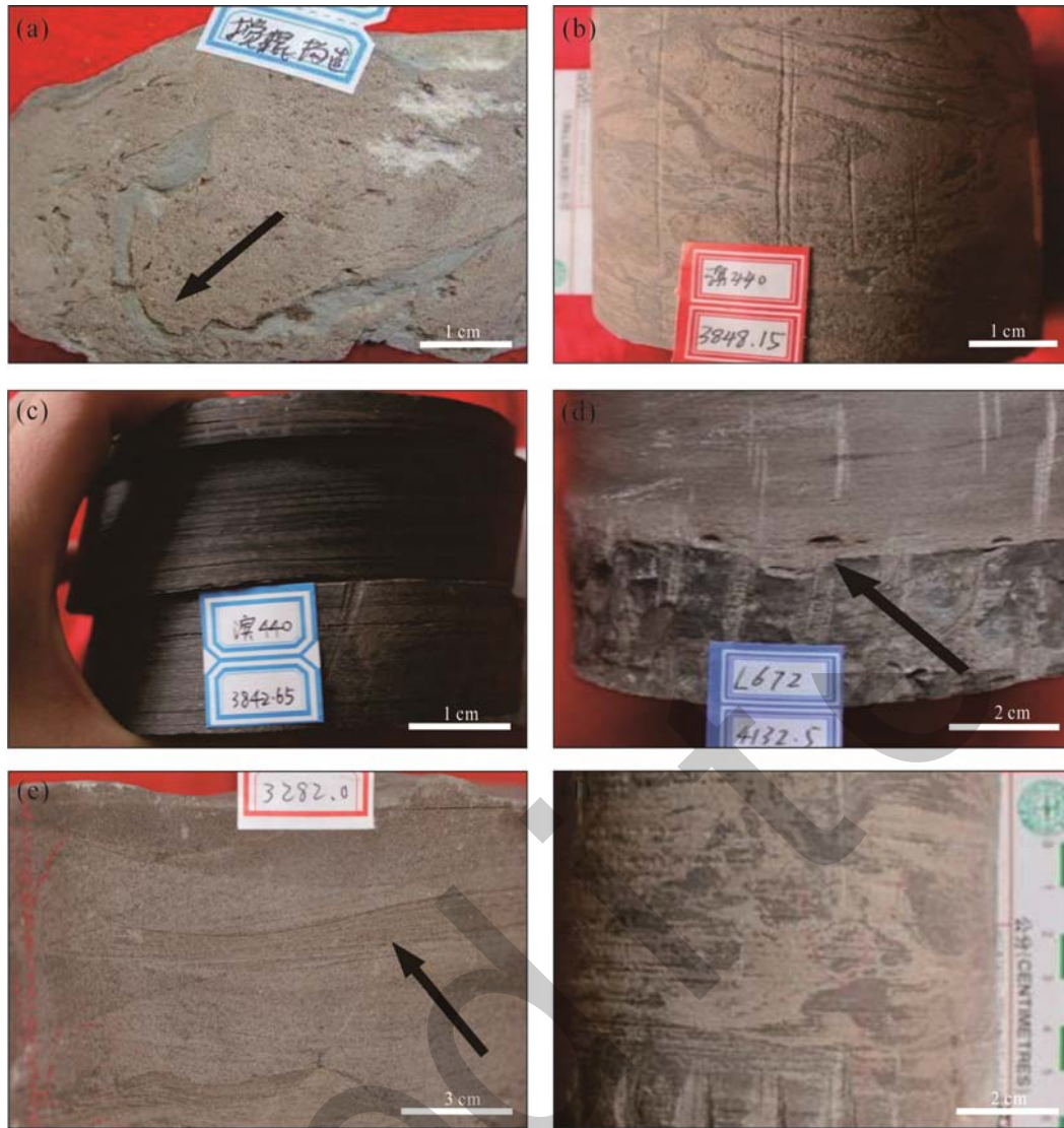
Figure 3. Cores of tempestite. (a): Well Bin 666, 3094.1m, "V" shaped tear shale cuttings; (b): Bin 440, 3848.15m, rumbled structure; (c): Bin 440, 3842.65m, dark gray mudstone; (d): Li672, 4132.5m, gutter cast; (e): Bin 670, 3282m, hummocky bedding; (f): Bin 440, 3918.3m, mix structure.
