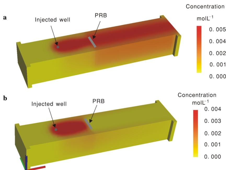
**Figure 2** Solute plumes 365 days after source injection: a) conservative tracer; b) amount of nitrate removed by the ZVI after crossing the PRB model with the updated rate
