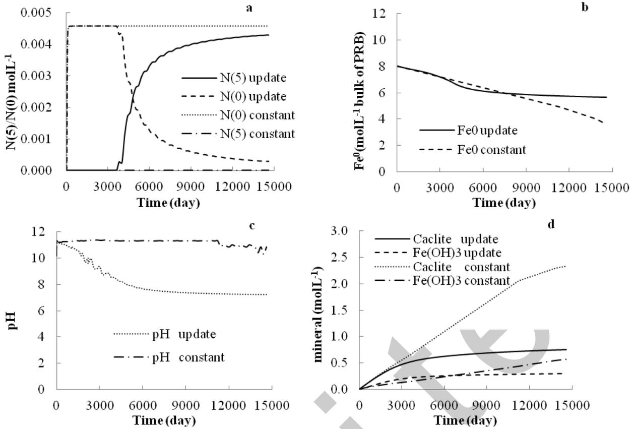
**Figure 3** Simulation results obtained using both models at the effluent face of the PRB (entrance face for secondary minerals) in the third layer over an operation time of 40 years: (a) nitrate and nitrogen, (b) ZVI, (c) pH, and (d) secondary minerals
