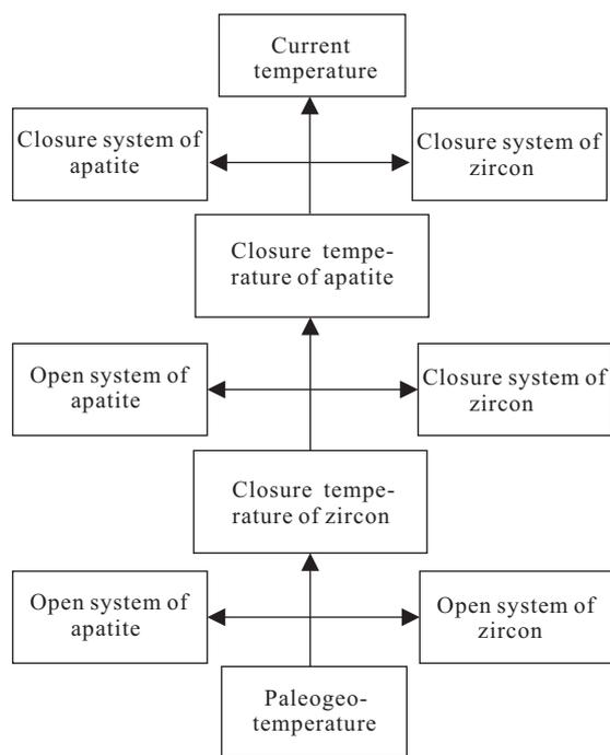
**Figure 1. The U-Th/He dating system and clock effect of apatite and zircon.**
