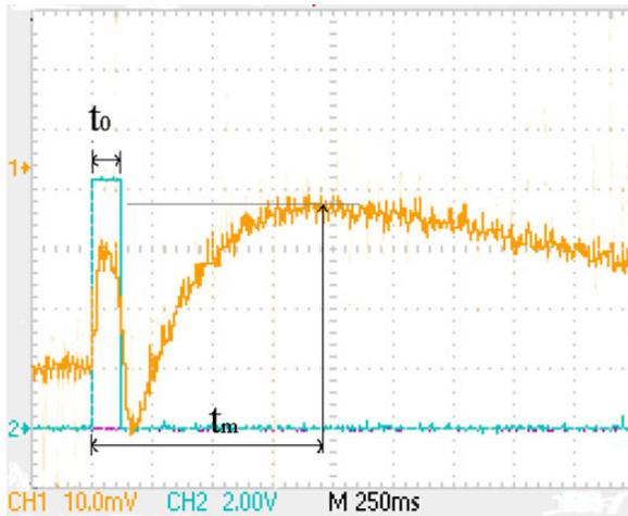
**Figure 2.** An input pulse and temperature response recorded using the oscilloscope (pulse length  $t_0=120$  ms,  $t_m=950$  ms. The horizontal scale interval time is 250 ms, the unit on the vertical is 10.0 mV for CH1 channel, 2.00 V for CH2 channel).
