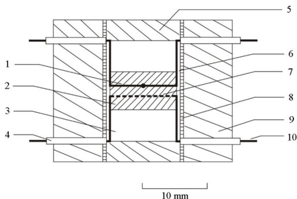
**Figure 1.** Schematic drawing of the sample assembly for measuring the thermal diffusivity at high temperature and pressure. 1. Thermocouple; 2. sample; 3. MgO block; 4. MgO sleeve; 5. Pyrophyllite space; 6. Al<sub>2</sub>O<sub>3</sub> sample tube; 7. impulse heater; 8. heater; 9. pyrophyllite; 10. lead.
