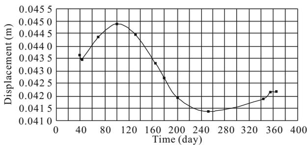
Figure 10. X displacement curve with water-level fluctuation at Node 238.
