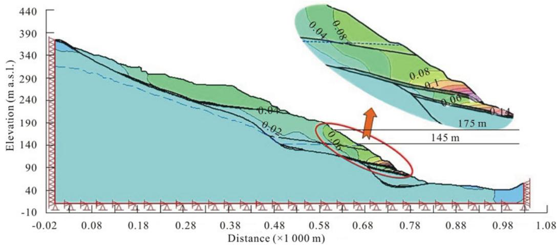
Figure 5.  $X$ -displacement contour of landslide under reservoir water-level 145 m.
