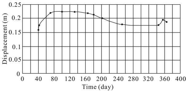
Figure 8. X displacement curve with water-level fluctuation at Node 123.
