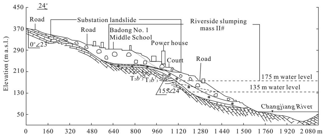
Figure 2.  $v-v'$  geological profile of Huangtupo landslide.
