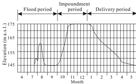
**Figure 4. Reservoir water-level running curve.**
