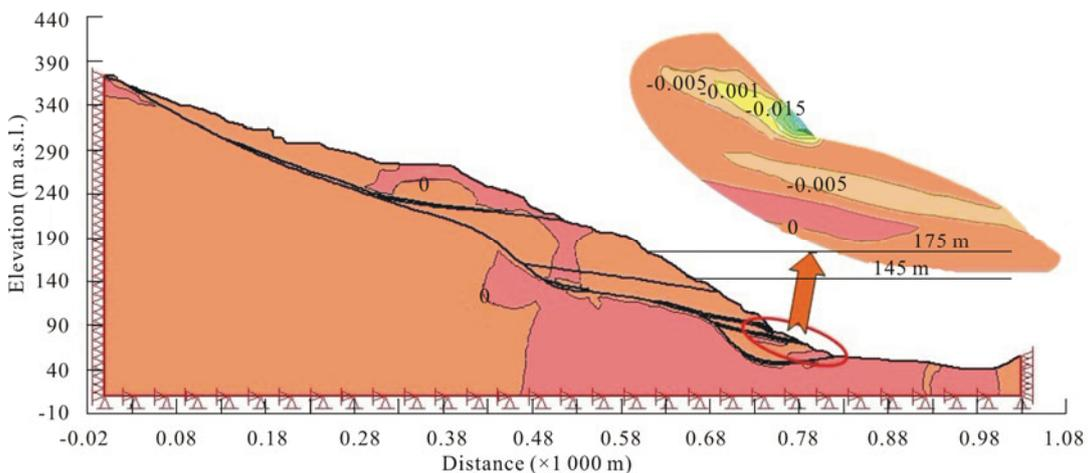
Figure 6.  $X$  strain contour of landslide under reservoir water-level 145 m.
