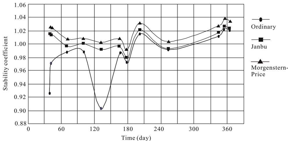
**Figure 11. Stability coefficient of riverside slumping mass II# changing with water-level fluctuation.**
