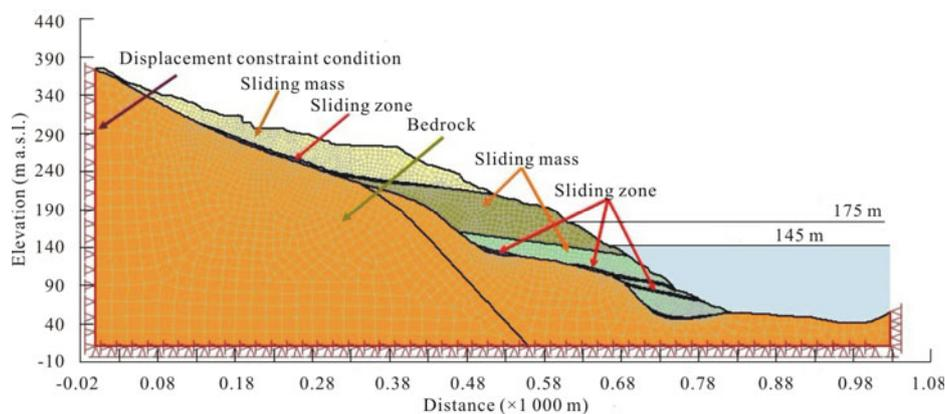
Figure 3. 2D numerical simulation meshes.
