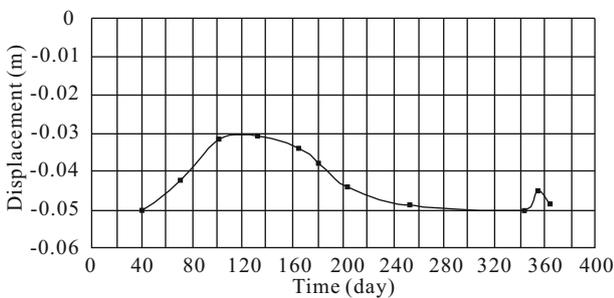
Figure 9. X displacement curve with water-level fluctuation at Node 191.
