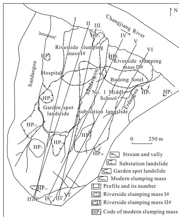
Figure 1. Engineering geological plan of Huangtupo landslide.
