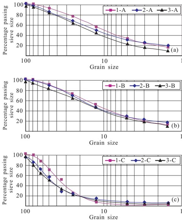
**Figure 2. Grading curves of the test sites. (a) The upper test sites; (b) the central test sites; (c) the bottom test sites.**
