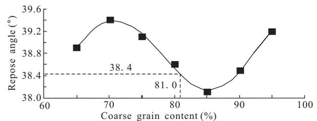
**Figure 4.** Relationship curve of repose angle and coarse grain content.
