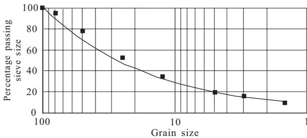
**Figure 3. Representative grading curve of coal gangue in Dongkuang.**
